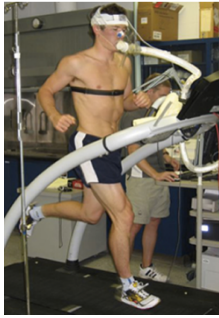
Figure 1: Example of a gold standard VO 2 max measurement using a treadmill, a metabolic cart, a chest strap HR monitor and a gas mask.
